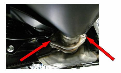
and the 15 MM socket and 15 MM wrench to loosen bolt at the upper mounting point on the frame
